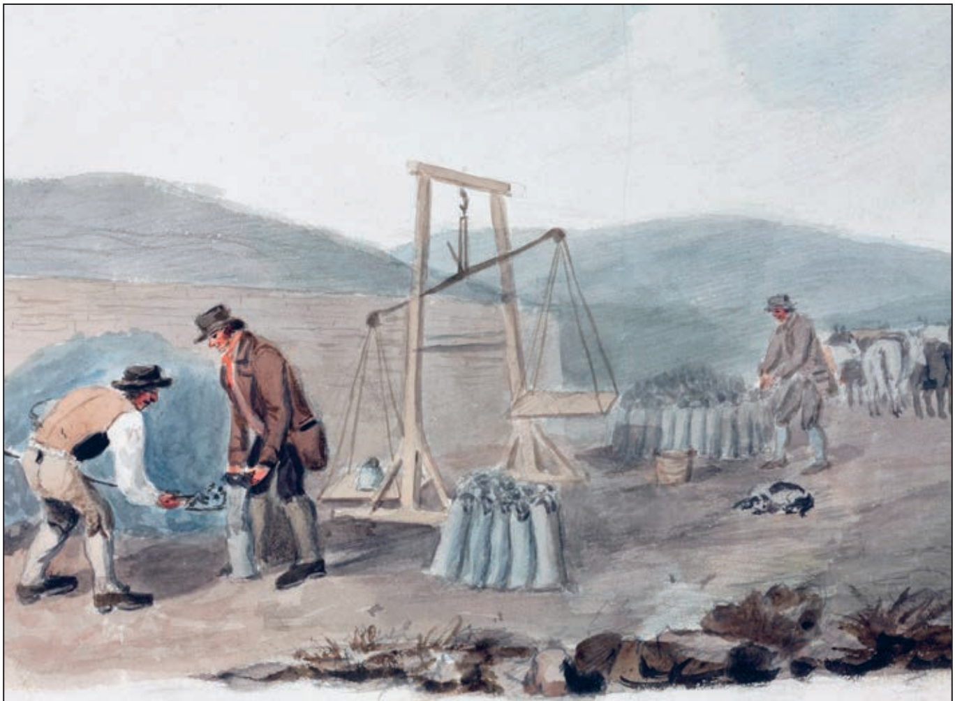
Figure 11. Weighing the lead concentrate and placing it into bags for transportation by mule to the smelter. This early nineteenth century scene from the North-East Pennines would have been repeated on the lead mines of County Wicklow. Reproduced by kind permission of the Science Museum
