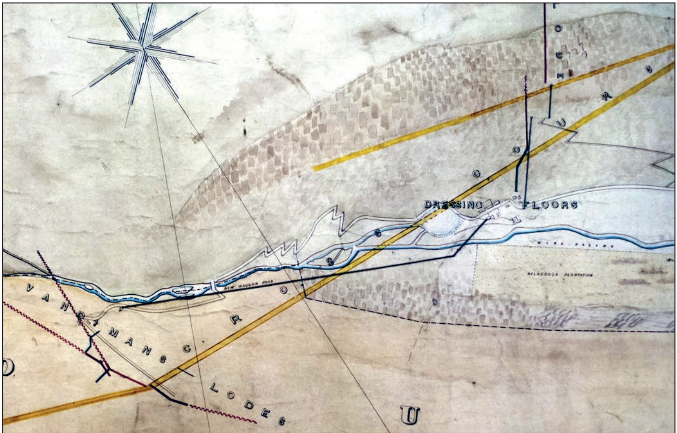
Figure 13. Section of a MCI map dated 1868, drawn by Captain G.J. Bailey. The inclined tramway from Van Diemen's Land depicted as a black line, can be seen running almost parallel to the Glenealo River from a drumhouse and waterwheel before turning left towards the Cornish rolls crusher house. The inclined tramways from the cliff portals of First and Second Adits may also be seen top right (as two black lines one above the other) heading towards the primary dressing floor
