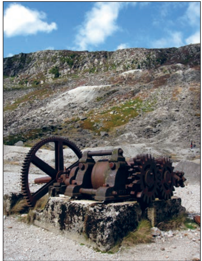
Figure 24. Cornish rolls crusher manufactured by John Mills of the Railway Foundry, Llanidloes, Wales. This is the finest crusher of its type in Ireland
