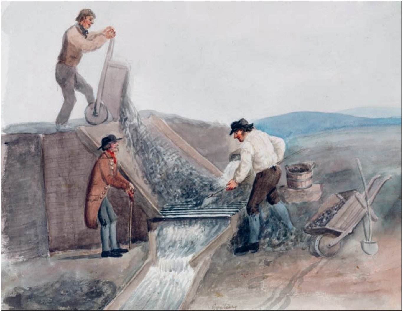
Figure 1. Grating lead ore in the North-East Pennines c.1805-1820. Reproduced with kind permission of the Science Museum
