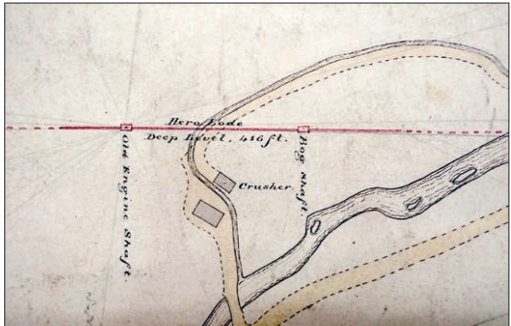
Figure 9. Section of a MCI mine plan dated July 1846 showing the Old Hero dressing floor which is located in the townland of Camaderry (otherwise known as Seven Churches). Note the leat bringing in water to feed the Cornish rolls crusher, housed in the rectangle on the right. The rectangle on the left is the 'mine yard'
