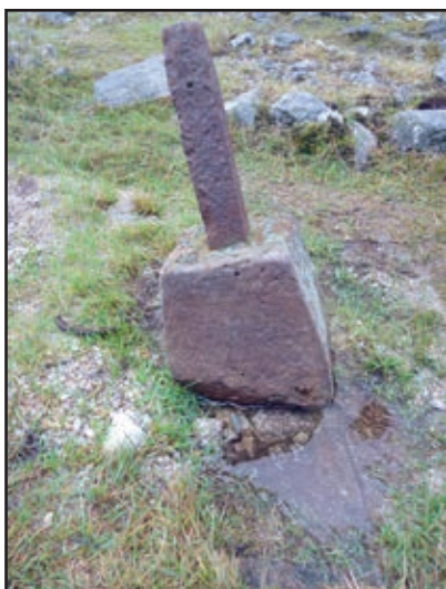
Figure 8. A well-worn short shank stamp shoe found in the vicinity of Luanure Adit where there was an early dressing floor. See the Perran Foundry Catalogue for similar examples (Trevithick Society 1986, p.13)
