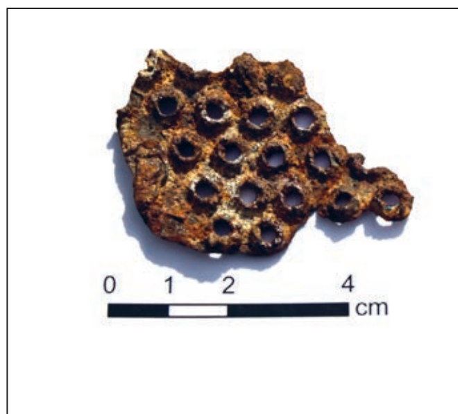
Figure 30. A fragment of stamp screen manufactured from punched iron sheeting, with holes approximately 3 mm (one eighth of an inch) in diameter
