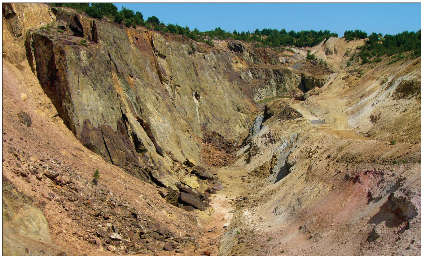
Fig. 16: A dramatic view down into the Cronebane Pit, East Avoca. Note entrances into old workings high up in the rock face. This, and the East Avoca Pit, offer unique opportunities to view exposures of volcanogenic sulphide mineralisation and are the best examples in Ireland of a cross section of a supergene or gossan zone of an oxidised orebody. The range of colours and unusual topography has attracted artists and film makers. Image, Martin Critchley, July 2005
